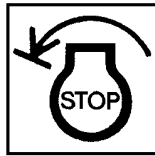
Stop control (on engine)
